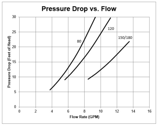
Figure 10-2: System Curve w/ 50 Equivalent ft. of Piping
