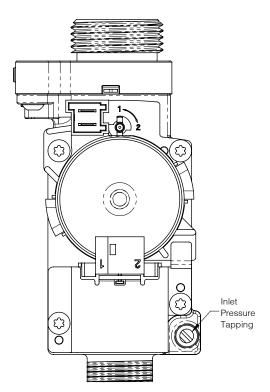
Figure 14-8: Gas Valve Inlet Pressure Tap
