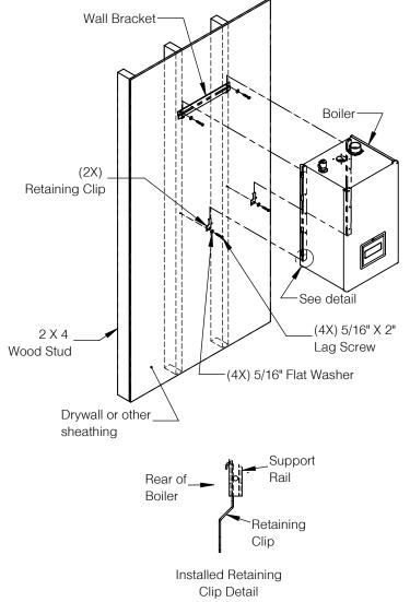
Figure 6-4: Mounting Boiler on Wall
