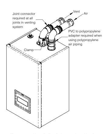
Figure 7-18: Near Boiler Polypropylene Venting
