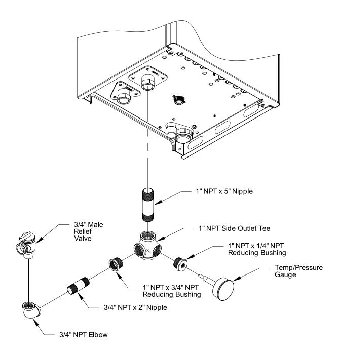
Figure 10-5: Near Boiler Piping Supplied with Boiler
