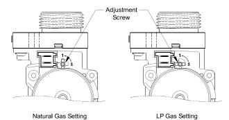
Figure 14-2: Gas Valve Fuel Setting
