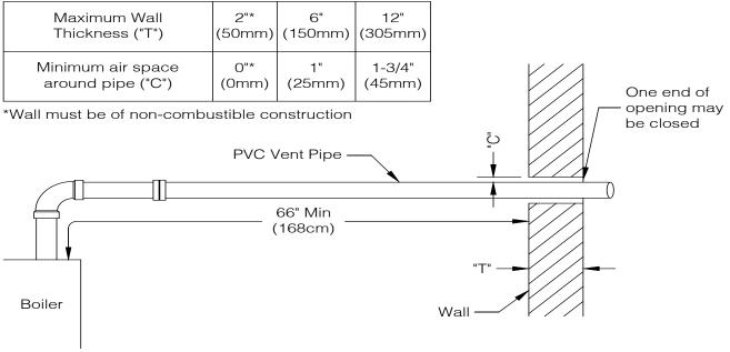
Figure 7-14: PVC Venting Wall Penetration Clearance
