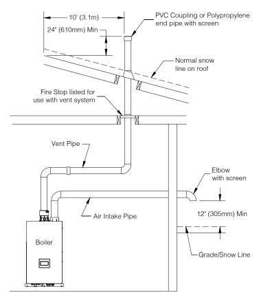
Figure 9-5: Alternate Vertical Vent/Sidewall Air Terminal
