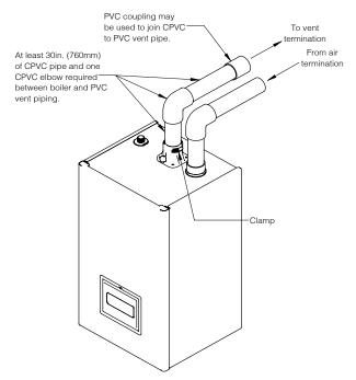
Figure 7-12: Near Boiler CPVC/PVC Venting
