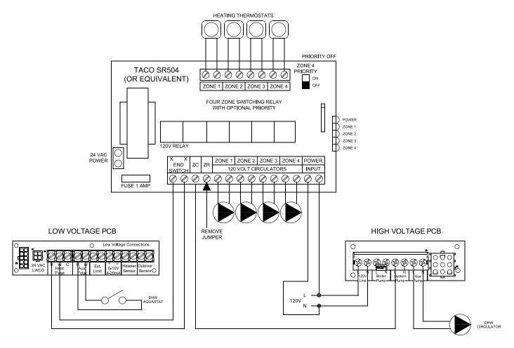
\*\*\*USE SAME POWER SOURCE FOR ALL CONTROLS AND ENSURE POLARITY TO ALL CONTROL DEVICES IS CORRECT
