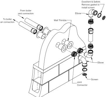
Figure 8-6: Polypropylene Fittings Terminal Assembly
