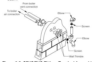
Figure 8-5: CPVC/PVC Fittings Terminal Assembly
