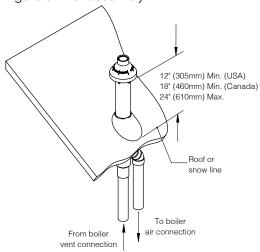
Figure 9-6: CPVC/PVC Concentric Terminal
