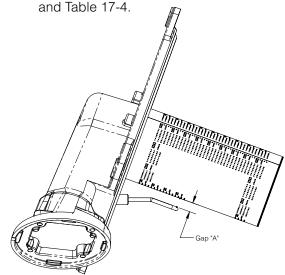
Figure 17-3: Ignitor/Flame Sensor to Burner Gap
