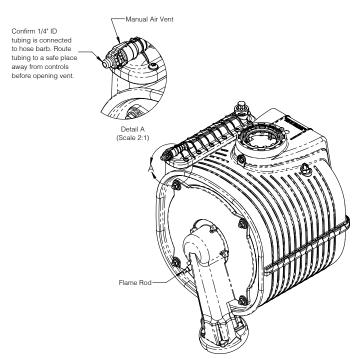
Figure 14-1: Manual Air Vent Location
