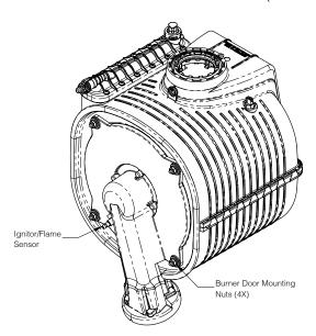
Figure 17-1: Ignitor/Flame Sensor Location
