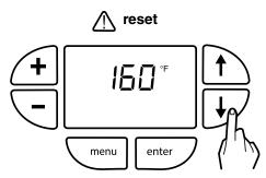
Figure 15-3: Viewing boiler status
