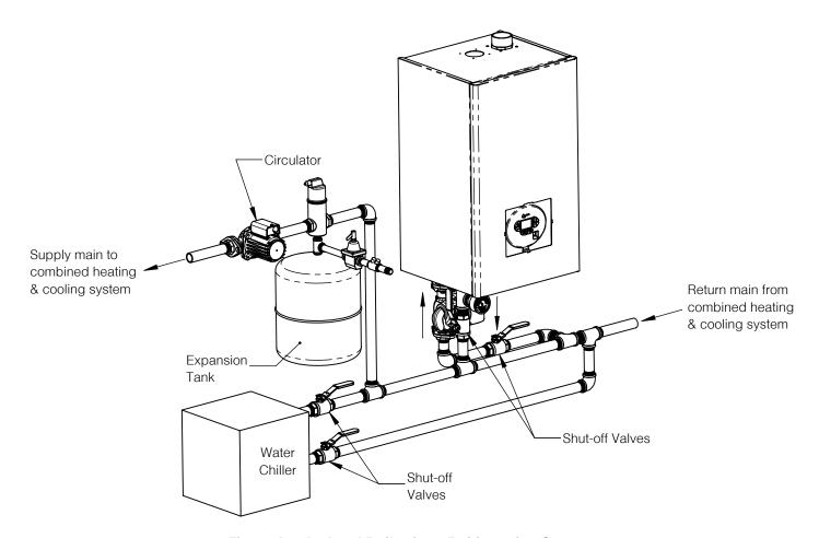
Figure A-1: Isolated Boiler from Refrigeration System
