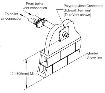
Figure 8-14: Polypropylene Concentric Terminal
