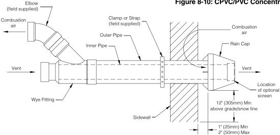
Figure 8-11: CPVC/PVC Concentric Terminal Installation
