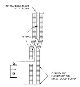
Figure 9-17: Masonry Chimney Chase Requirements
