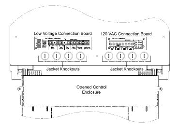
Figure 12-1: Location 120 VAC and Low Voltage Connection Boards
