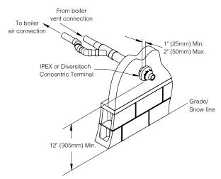
Figure 8-10: CPVC/PVC Concentric Terminal
