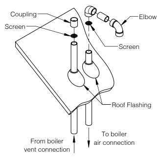
Figure 9-3: CPVC/PVC Fittings Terminal Assembly
