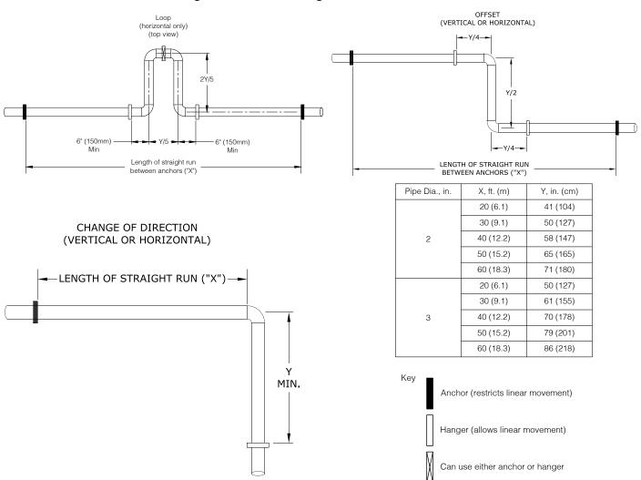
Figure 7-15: CPVC/PVC Venting Expansion Loops
