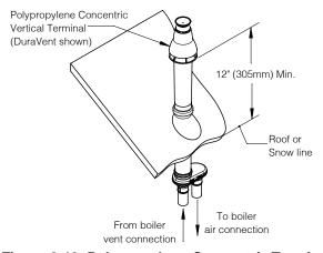
Figure 9-10: Polypropylene Concentric Terminal
