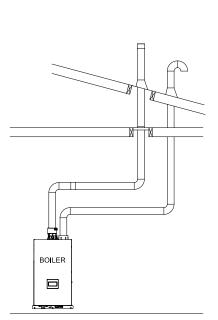
Figure 7-4: Vertical Termination with Fittings see Section 9 for details
