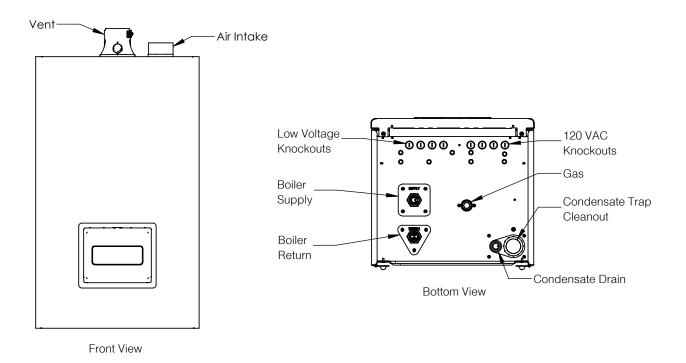
Figure 3-6: Boiler Connections
