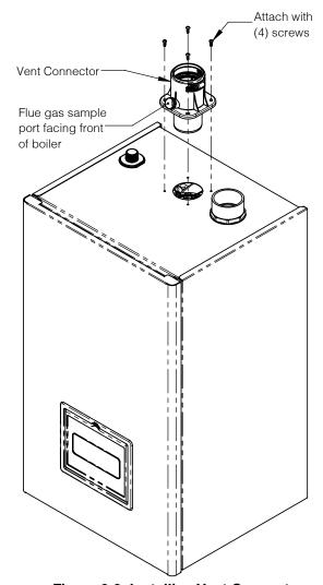
Figure 6-2: Installing Vent Connector
