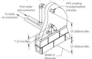
Figure 8-4: Alternate Fittings Terminal
