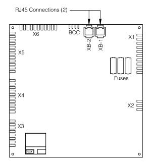
Figure 12-4: Boiler-to-Boiler Connections
