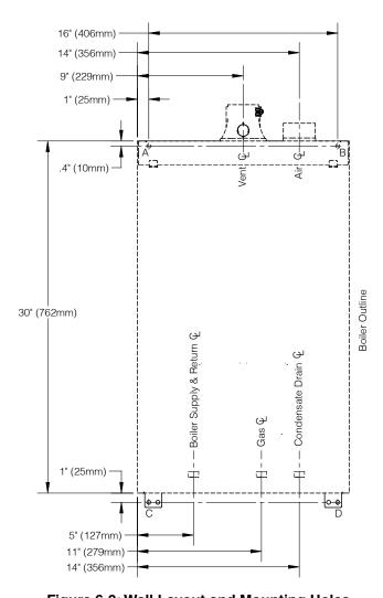
Figure 6-3: Wall Layout and Mounting Holes
