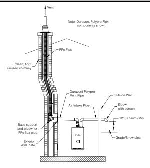
Figure 9-16: Masonry Chimney Chase System
