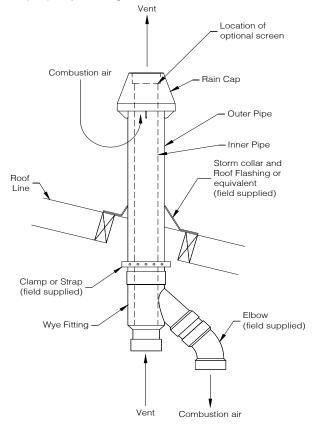
Figure 9-7: CPVC/PVC Concentric Vertical Installation
