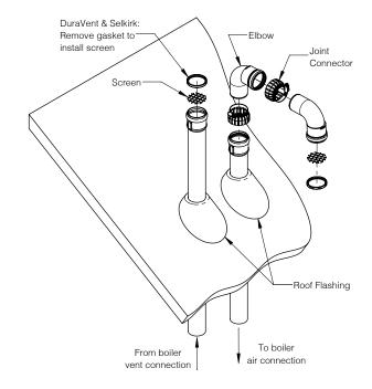
Figure 9-4: Polypropylene Fittings Terminal Assembly
