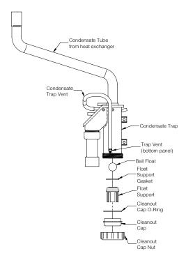
Figure 17-5: Condensate Trap Exploded Parts View
