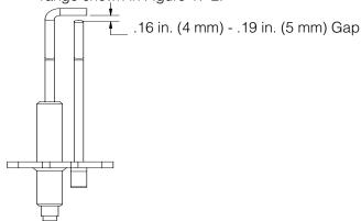
Figure 17-2: Ignitor/Flame Sensor Spark Gap
