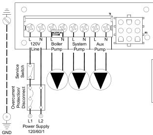
Figure 12-2: 120 VAC Connections
