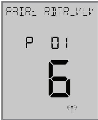
After 3 seconds, the AWRT10RF Thermostat will enter the parameter setup mode, starting with P 01 (displayed with RDTR\_VLV flashing). The number of radiator valves connected is also displayed.
