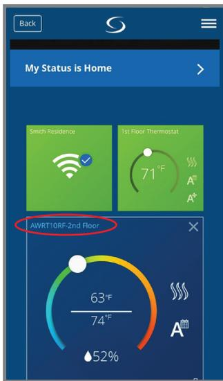
Choose the thermostat that controls the Radiator Valve Actuators. Then select the thermostat name (circled in red).
