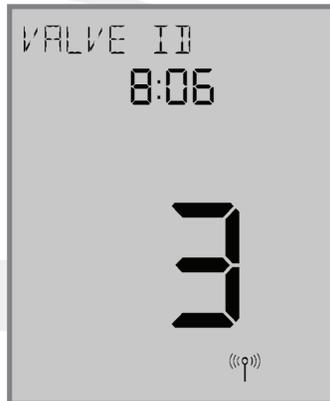
As each ARV/AVA Valve Actuator is paired with the AWRT Thermostat, the ID number displayed on the screen will increment.
