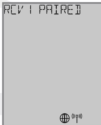
After pairing is complete, a confirmation screen is displayed on the AWRT10RF Thermostat for 3 seconds, then the device will enter the parameter setup mode.
