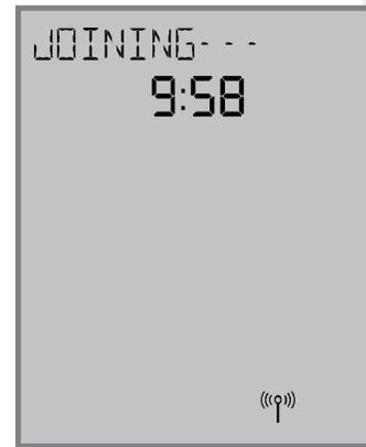
JOINING- - - is displayed with a 10 minute countdown timer to show the remaining time available to complete the next steps. The  $\text{((\text{P}))}$  icon will flash at the bottom of the screen indicating that the thermostat is searching for a network to join.
