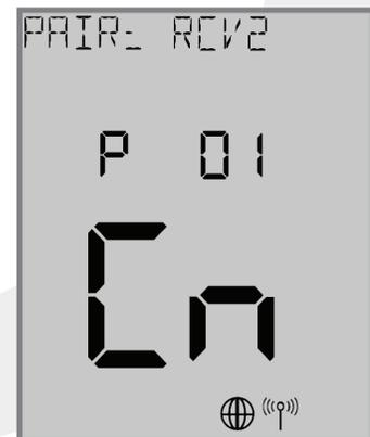
The thermostat display will show PAIR: RCV2 with P 01 indicating it is in the parameter setup mode. Cn (Connected) indicates that the AX10RF Receiver is paired and connected.
