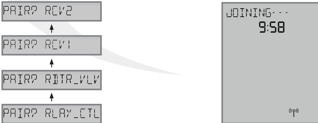
**Step 1.** On the AWRT10RF Thermostat, press ^ until PAIR? RCV2 is displayed. Press SELECT.
