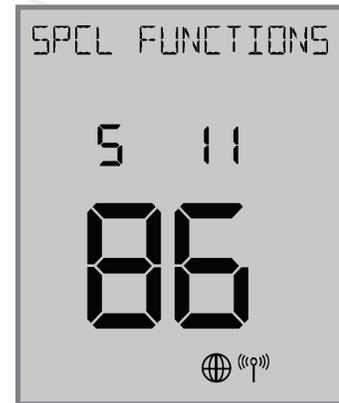
**Reset to Factory Settings:** To reset the AWRT10RF Thermostat to factory settings, change the S 11 value to "86" and choose "Y" to reset.
