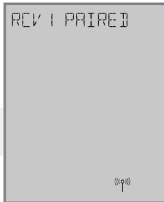
After pairing is complete, a confirmation screen is displayed for 3 seconds, the AWRT10RF Thermostat enters the parameters set up mode.
