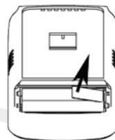
**Step 6.** Remove the battery tab to power the AWRT10RF Thermostat
