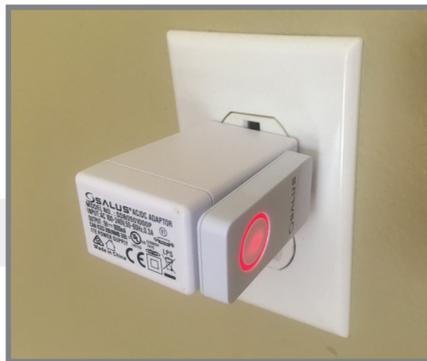
**Step 1.** Press and hold the lighted red button on the AC10RF Coordinator for 5 seconds until the LED begins flashing, to begin pairing. When the network status LED on the AKL Relay Controller and the backlight on the Auto/Manual switch of the AX10RF (if used) stop flashing, they have joined the network and you are ready to pair the AWRT Wireless Radiant Thermostat.
