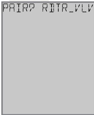
**Step 4.** Use the  $\wedge$  and  $\vee$  keys on the AWRT10RF Thermostat to switch from RLAY\_CTL to RDTR\_VLV. Press SELECT to initiate pairing.
