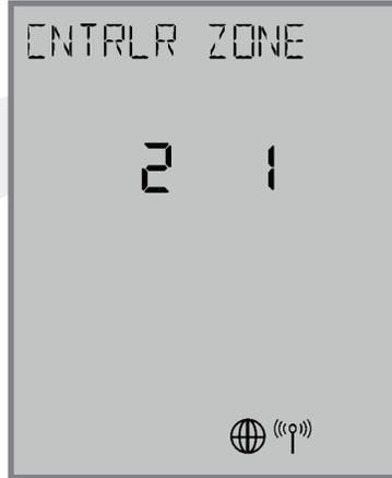
**Step 8.** Use the  $\wedge$  and  $\vee$  keys to change the CONTROLLER value, then the  $\lt$  or  $\gt$  key to switch to the ZONE.
