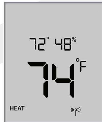
**Step 2.** Press the ^ or v keys to adjust the target setpoint. The new setpoint will take effect once the display stops flashing.
