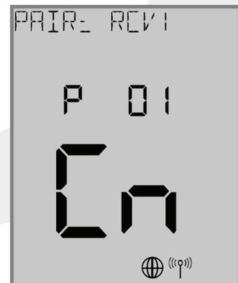
The thermostat display will show “PAIR: RCV1” with P 01 indicating it is in the parameter setup mode. “Cn” (Connected) indicates that the AX10RF Receiver is paired and connected.
