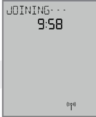
JOINING- - - is displayed with a 10 minute countdown timer to show the remaining time available to complete the next steps. The  $\langle\langle\circ\rangle\rangle$  icon will flash at the bottom of the screen indicating that the thermostat is searching for a network to join.
