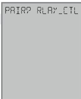
**Step 1.** If PAIR? RLAY\_CTL is not displayed and flashing, use the  $\wedge$  or  $\vee$  keys to display it. Press the SELECT key on the AWRT10RF Thermostat.
