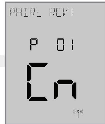
The display will show PAIR: RCV1 with P 01 indicating it is in the parameter set up mode. Cn (Connected) indicates that the AX10RF Receiver is paired and connected.
