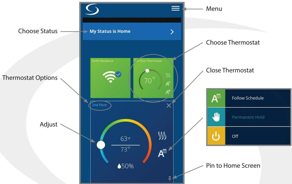
**Thermostat Options:** Press Thermostat Options to advance to the screen below.
