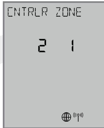
**Step 4.** Use the  $\wedge$  and  $\vee$  keys to change the CONTROLLER value, then the  $\lt$  or  $\gt$  key to switch to the ZONE.
