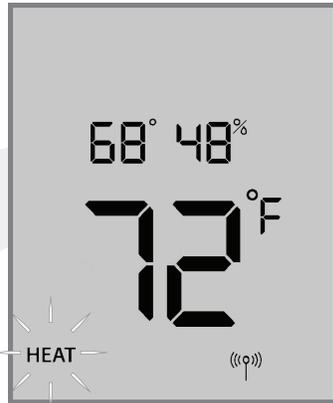
The new mode setting will flash and the current setpoint temperature will appear above the room temperature display. If the mode is OFF, the setpoint will change to 41°F (5°C).
