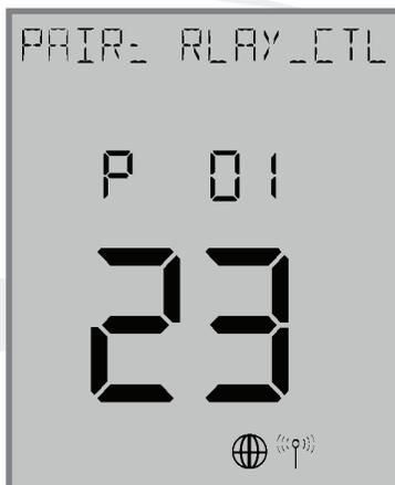
The AWRT10RF Thermostat will enter parameter setup mode, starting with parameter P 01. The current device type along with the Zigbee channel number will be displayed.
