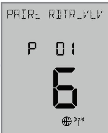
In parameter setup mode, the AWRT10RF Thermostat starts with P 01 (displayed with RDTR\_VLV flashing)
