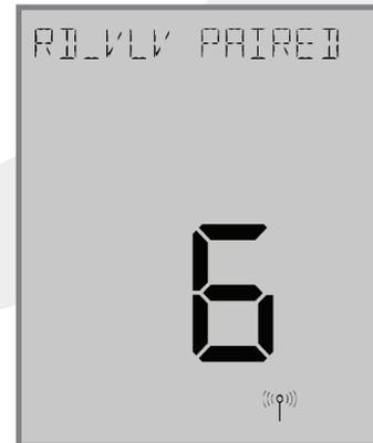
If the user presses the  $\odot$  key, the timer times out or 6 valves have been paired, the display will read "RD\_VLV PAIRED" for 3 seconds.
