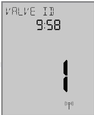
The AWRT Thermostat will display the Valve ID number and a 10-minute timer showing how much time is left to finish pairing.
