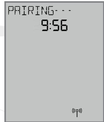
**Step 5.** Use the  $\wedge$  and  $\vee$  keys to change the ZONE value, then press SELECT. The AWRT10RF Thermostat will then display PAIRING-- as it associates with the selected controller and zone.
