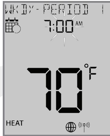
**Step 6.** Use the  $\wedge$  and  $\vee$  keys to change the minute to begin the first period. Press SELECT.
