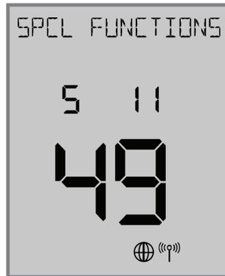
**Time/Date Functions:** If S 02 through S 10 are not accessible, change the S 11 value to "49" on the display using the ^ or v keys and press enter. Change item P02 to YES to enable thermostat programming.
