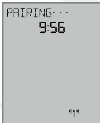
Once the AWRT10RF Thermostat joins a network, the
