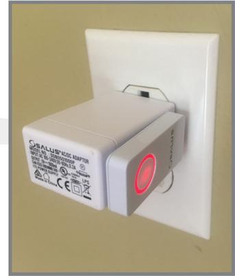
**Step 5.** Press & hold the flashing red pairing button on the AC10RF Coordinator for 5 seconds to complete the pairing process.
