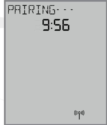
**Step 9.** Use the  $\wedge$  and  $\vee$  keys to change the ZONE value, then press SELECT. The AWRT10RF Thermostat will then display PAIRING-- as it associates with the selected controller and zone.
