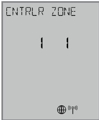
When the AWRT10RF Thermostat has found all controllers in the network, it will display the default relay controller value (1) and the default zone value (1). If there is more than 1 relay controller on the network, the left value CNTRLR will flash. If there is only one relay controller, the right-hand value for ZONE will flash.
