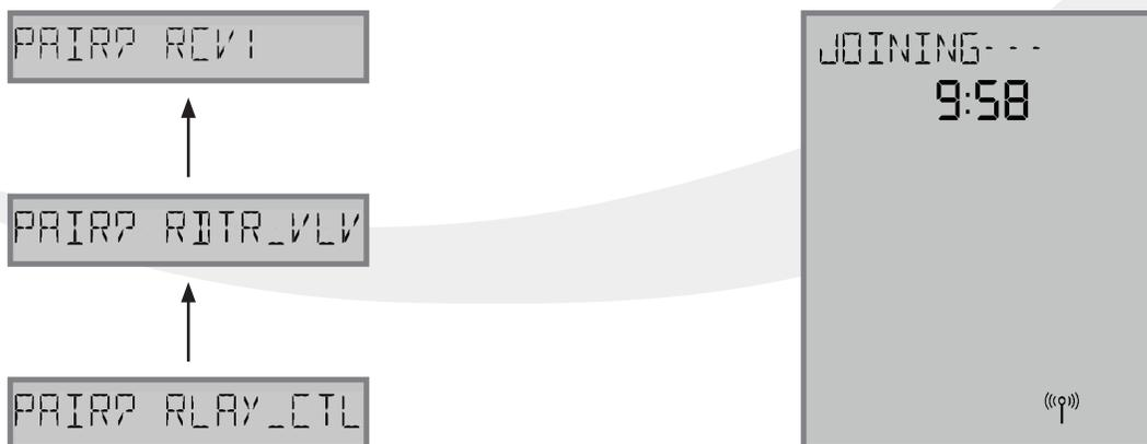
**Step 1.** On the AWRT10RF Thermostat, press  $\wedge$  until PAIR? RCV1 is displayed. Press SELECT.
