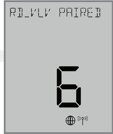
If the user presses the
