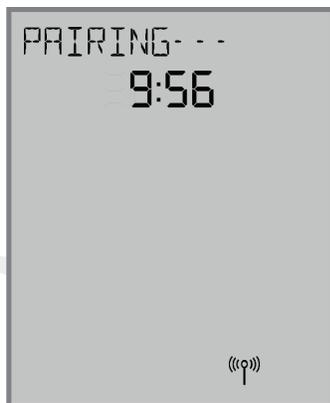
Once the AWRT10RF Thermostat joins a network, the
