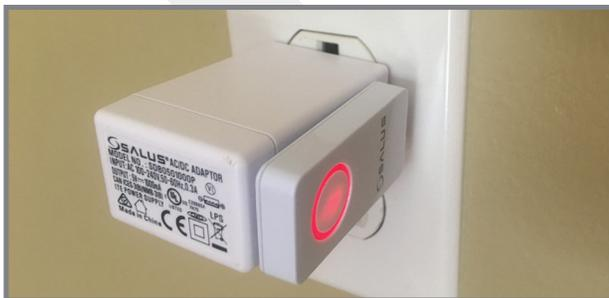
**Step 1.** Press and hold the lighted red pairing button on the AC10RF Coordinator for 5 seconds, until the LED begins to flash.
