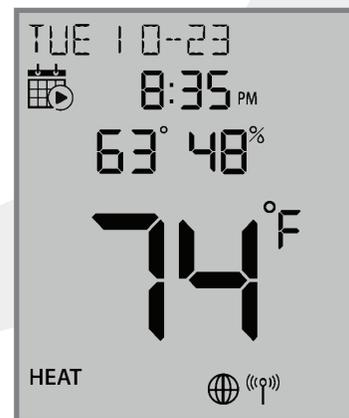
**Step 6.** Press the  $\odot$  key to exit parameter setup and go to the Home Screen. The display shows the current date & time, target temperature, relative humidity, network/internet status and room temperature.
