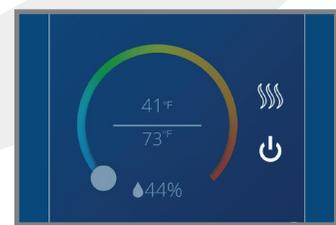
Pressing "Off" will cause the AWRT10RF Thermostat to stop calling for heat until it is turned back on.
