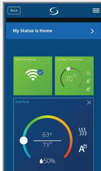
To change the current temperature setpoint, move the dial to the desired temperature.
