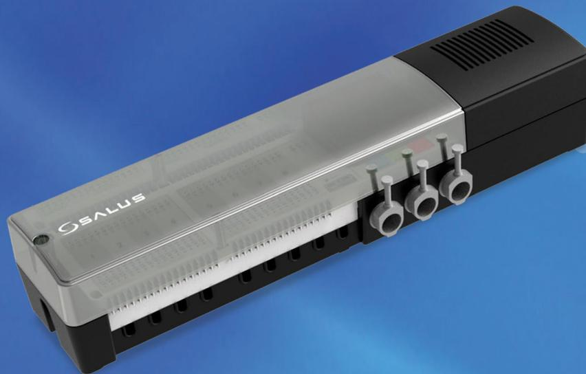
The SALUS AKL08 Relay Controller for underfloor heating systems is the perfect interface between thermostats and actuators. It ensures precise control for optimum comfort and efficiency. Volt-free connections for Pump and Boiler integration, 120 VAC power input, 24 VAC outputs, and Night Set Back control allow the AKL08 to fit any situation.
